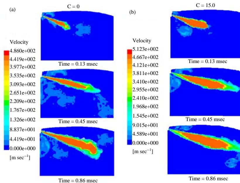
Fig. 4(a-b): (a) Contours of the spray tip velocity for the concentration ratios C = 0 and (b) 15% at different times after start of injection
