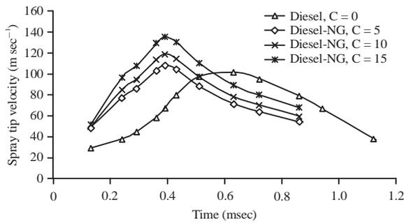
Fig. 5: Spray tip velocity of diesel and diesel-NG when the concentration of NG dissolved in diesel at C = 0, 5, 10 and 15%
