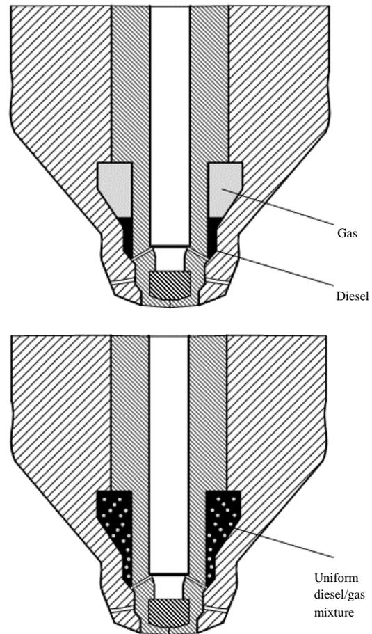
Fig. 1: A simplified representation of two methods of diesel-gas mixing within a co-injector gas plenum<sup>8</sup>
