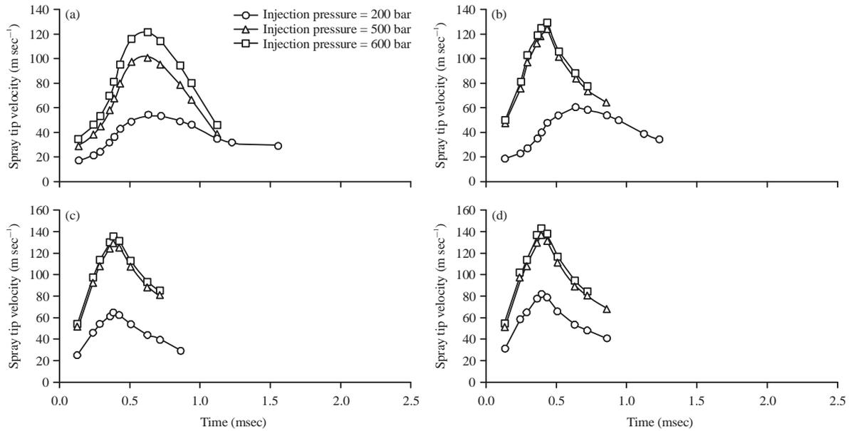
Fig. 8(a-d): Effect of different injection pressures (200, 500 and 600 bar) on spray tip velocity (a) C = 0, (b) C = 5.0%, (c) C = 10.0% and (d) C = 15%
