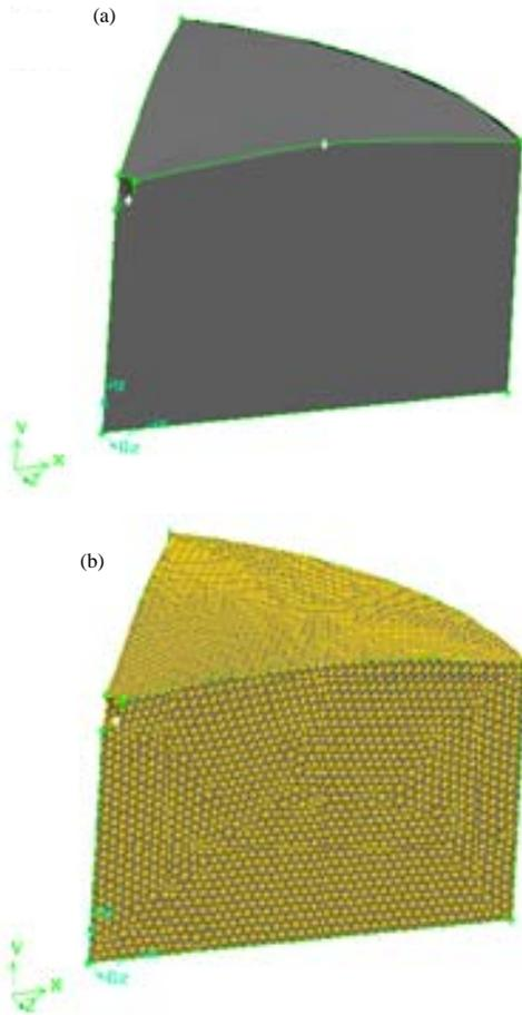
Fig. 3(a-b): (a) Solid modeling and (b) Mesh for case under study
