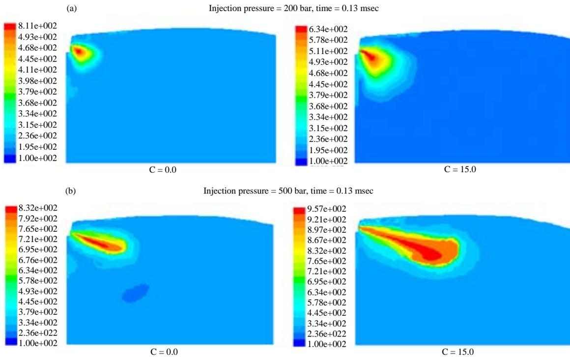
Fig. 7(a-b): (a) Contours of the diesel and diesel-NG dissolved at C = 0.0 and (b) 15 at injection pressure 500 bar
