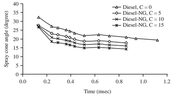
Fig. 6: Spray cone angle of diesel and diesel-NG at injection pressure: 500 bar of diesel-NG at C = 0, 5, 10 and 15%
