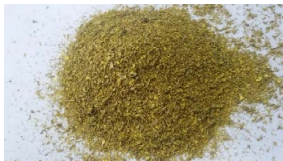
Fig. 1: Kinetic Degradation Fluxion (KDF) material using in filter
