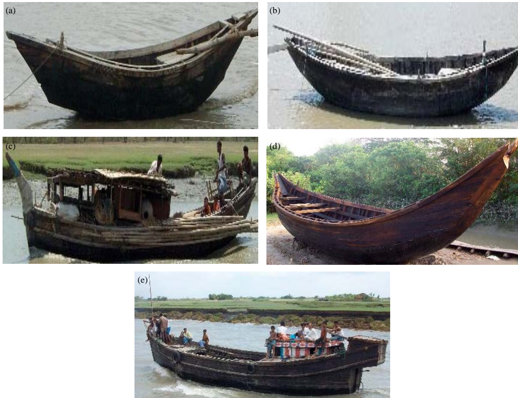
Fig. 2(a-e): Several crafts used for fishing in Hatiya island (a) Kosha nauka, (b) Dingi nauka, (c) Chandi nauka (d) Soto tempu and (e) Balam nauka
