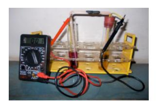
Fig. 1: Microbial fuel cell
