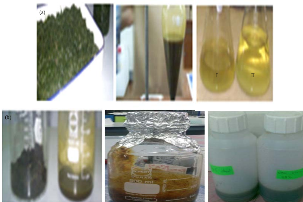
Fig. 1(a-b): (a) Oil extraction and biodiesel yield from algae and (b) Bioethanol production by fermentation bioprocess (algae) (oil extraction) biodiesel (I: single, II: mixture)
