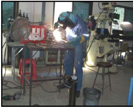
Fig. 6: Shield metal arc welding process
