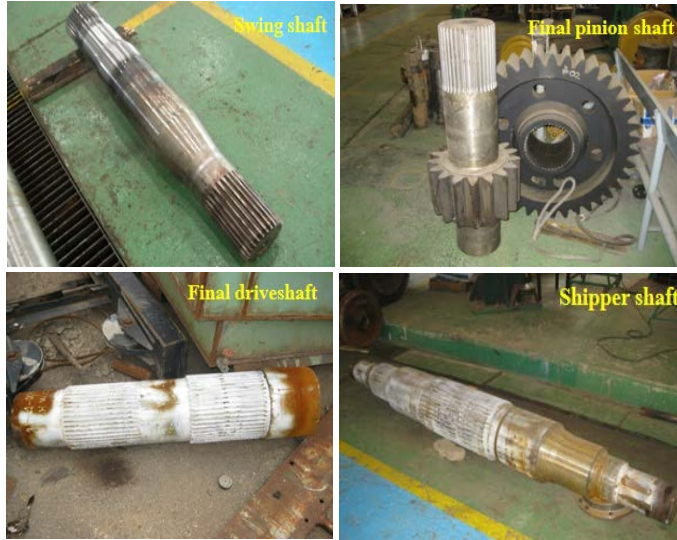
Fig. 1 The swing shaft in transmission system
