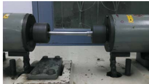
Fig. 10: Perform fatigue test
