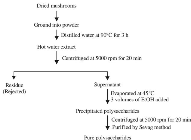
Fig. 2: Flow chart for the isolation and purification of polysaccharides
