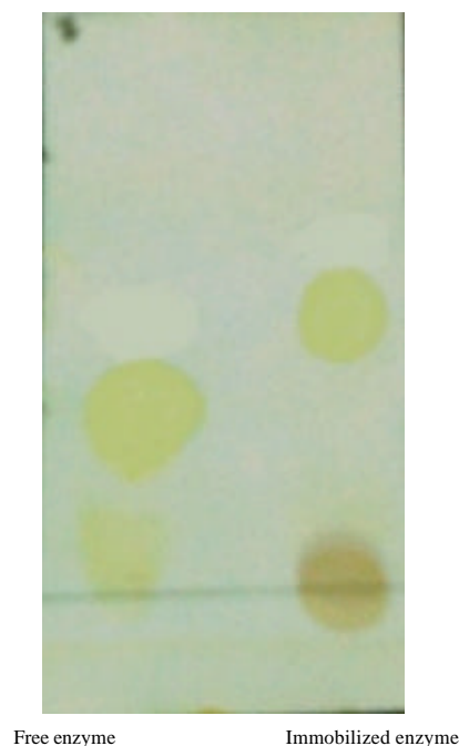
Fig. 8: Thin layer chromatography of biodiesel produced using free enzyme and immobilized enzyme as catalyst
