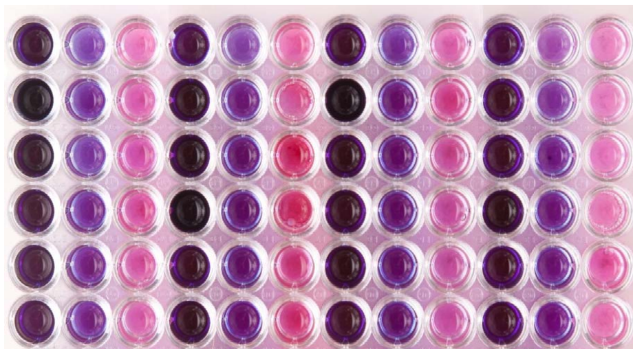
Fig. 1: Microtiter plate with three E. coli strains to demonstrate differential resazurin color change post X-irradiation
