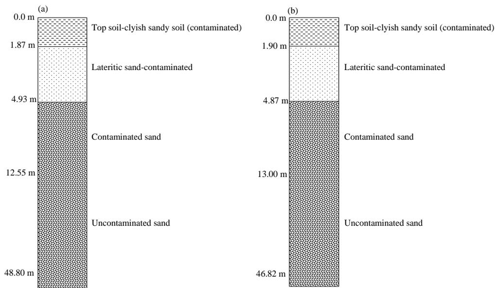
Fig. 6(a-b): Interpreted geoelectric sections for (a) VES A and (b) VES B
