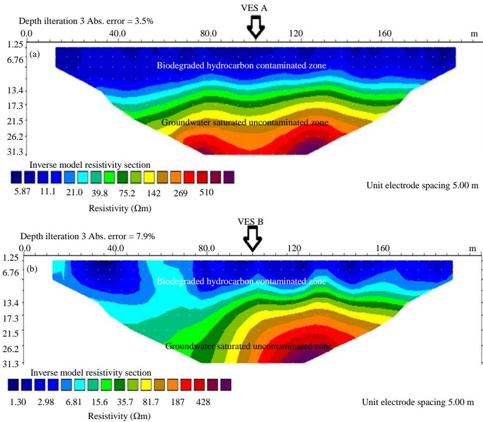
Fig. 4(a-b): ERT image site, (a) 1 along traverse A (27 months of spill) and (b) 2 along traverse B (42 months of spill), ERT: Electrical resistivity tomography and VES: Vertical electrical resistivity sounding
