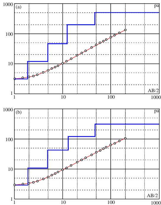
Fig. 5(a-b): AA curve types of interpreted (a) VES A and (b) VES B, VES: Vertical electrical resistivity sounding
