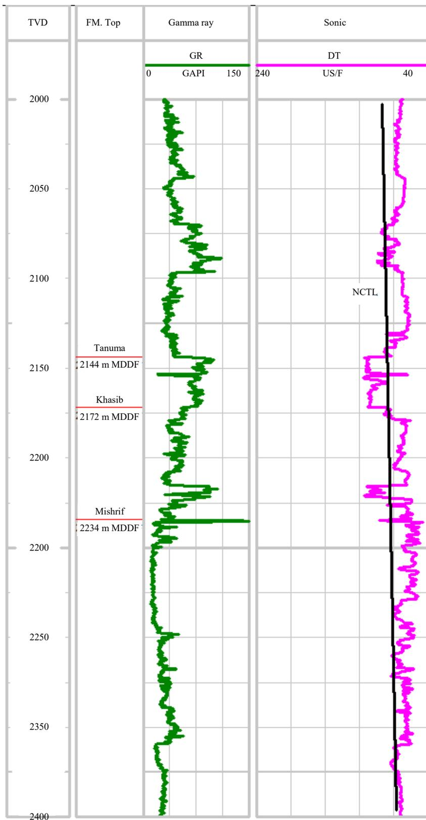
Fig. 5: NCTL on compressional sonic log in one of the studied wells from Zubair field, indicating Tanuma shale formation (2144-2172 m TVD) has higher porosity with respect to NCTL
