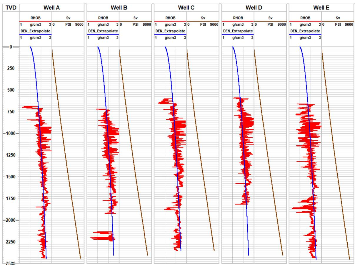
Fig. 3: Extrapolated density log (blue curve) to the surface, wireline density (red curve) and estimated vertical stress (brown curve) for the studied wells in Zubair field
