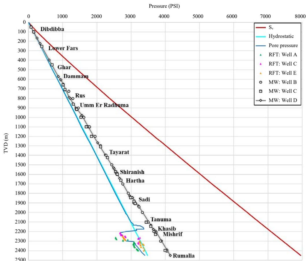
Fig. 7: Regional vertical stress, hydrostatic pressure and pore pressure profile for Zubair field along with formation tops, drilling mud weight and RFT measurements from five studied wells
