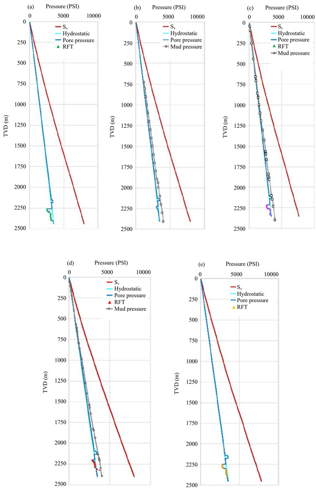
Fig. 6(a-e): Vertical stress, hydrostatic pressure and estimated pore pressure in (a) Well A, (b) Well B and (c) Well C (d) Well D and (e) Well E along with available mud weight and RFT data set
