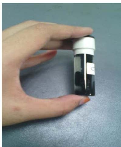
Fig. 1: Test on detection of SRB by sani test kit
