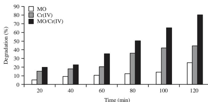
Fig. 5: Percent degradation of MO, Cr(VI) and MO/Cr(VI) Vs. time
