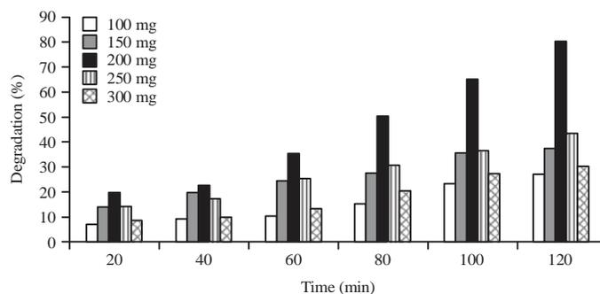
Fig. 4: Percent degradation of MO/Cr(VI) Vs. time by varying the amount of Sn/ZnO (100-300 mg)
