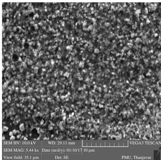
Fig. 2: SEM micrograph of Sn doped ZnO nanoparticles
