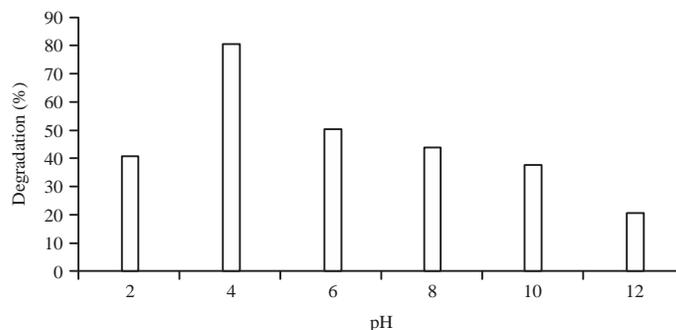
Fig. 6: Percent degradation of MO/Cr(VI) at 120 min by varying the pH of the solution keeping MO/Cr(VI) concentration and Sn/ZnO amount as constant
