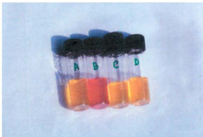
Fig. 1B: Urease test determine ammonia production A and C: Fresh medium color indicate negative result, B: Deep pink color indicates positive result, D: Negative control
