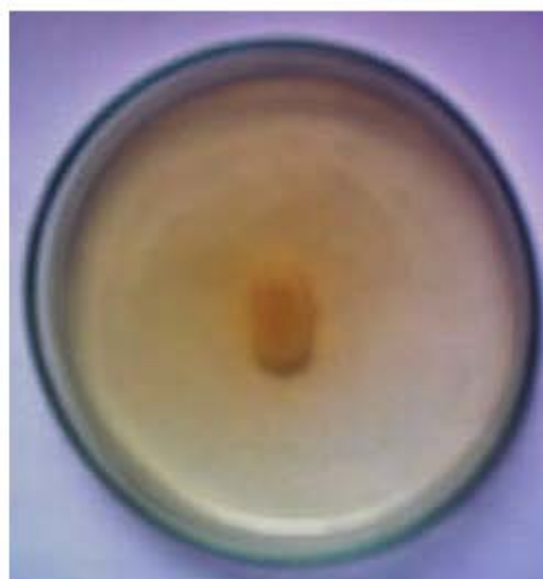
Fig. 5: Bacterial isolate RA-20 showing yellow coloration after 24 h of growth in minimal medium supplemented with 100 µg mL -1 of methyl parathion. Methyl parathion is degraded to p-nitrophenol by organophosphorus hydrolase
