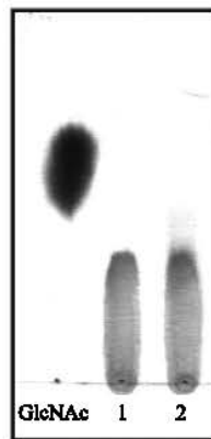
Fig. 7: Paper chromatogram of the hydrolysis product of pNP-N-acetylglucosaminide after incubation with chitinase crude enzyme. GlcNAc = N-acetylglucosamine as standard, lane 1 = the enzyme was incubated with the substrate for 2 h at 37°C. Lane 2 = the enzyme was incubated with the substrate for 5 h at 37°C
