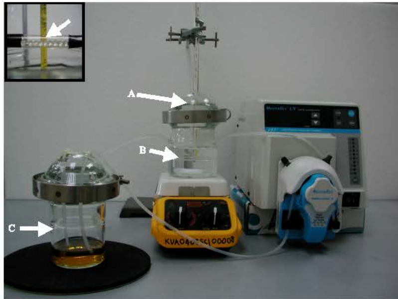
Fig. 1: NAM model (A) inside the water bath (incubator) (B) connected to a reservoir (C) via a peristaltic pump. Inset is the enlarged picture of A (indicated by the arrow)
