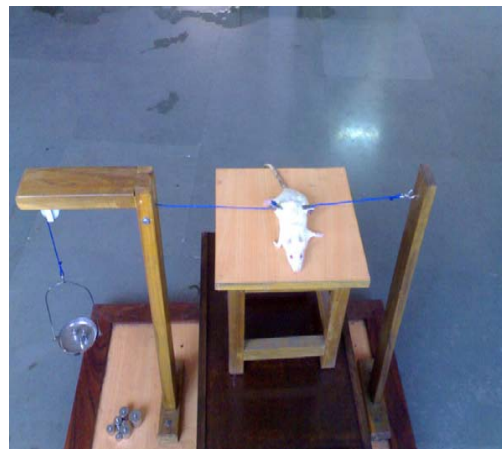
Fig. 4: Tensiometer for the measurement of tensile strength of skin
