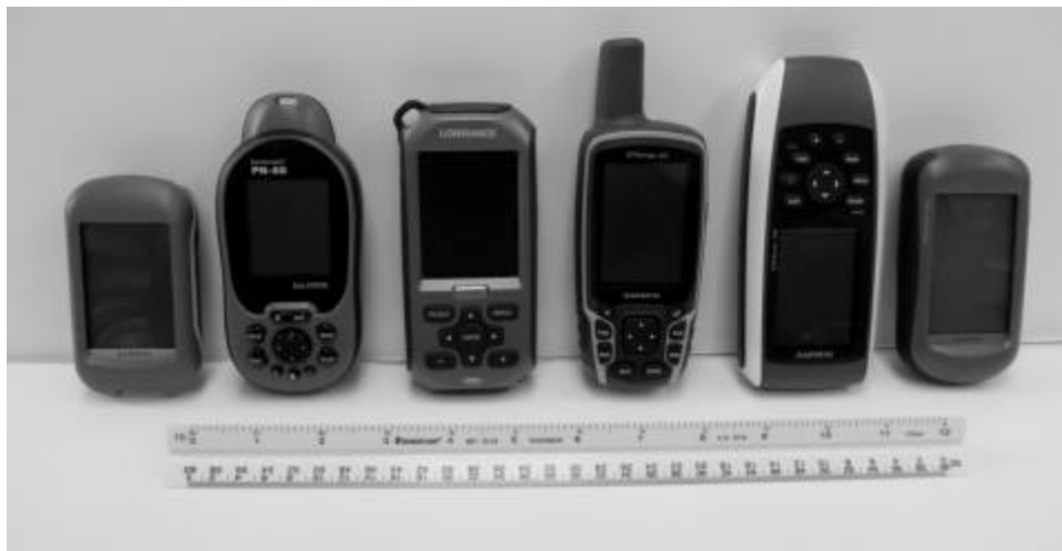
Fig. 1: Consumer-GPS receivers involved in measurement testing: Dakota 10, Earthmate PN-60 Endura Sierra, GPSMAP 62, GPSMAP 78 and Oregon 450
