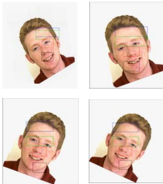
Fig. 9: Failure in detecting and correcting rotations of -25, -20, +20, +25 degrees from right to left respectively. Stirling University database (resized samples)
