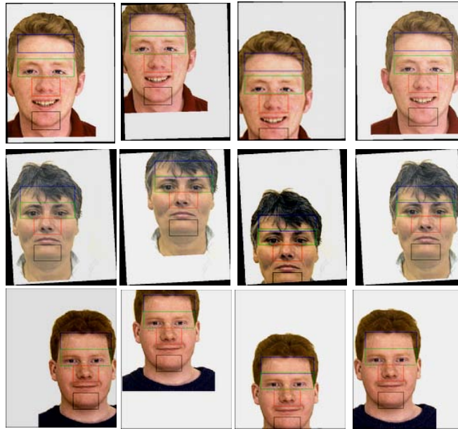
Fig. 6: Successfully locating and defining the face in different translation positions, from left to right, respectively: left, up, down and right translations. Stirling University database (resized samples)
