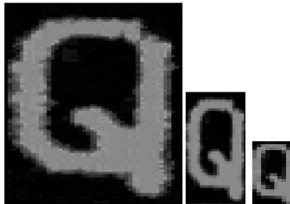
Fig. 4: The pyramid representation of a region of interest having the same number of levels as in Fig. 3
