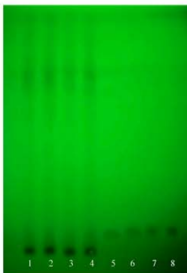
Fig. 2: Image of HPTLC plate (254 nm). 1: 5 \mu L Acetone extract (5 mg mL -1 ), 2: 10 \mu L acetone extract (5 mg mL -1 ), 3: 5 \mu L methanol extract (5 mg mL -1 ), 4: 10 \mu L methanol extract (5 mg mL -1 ), 5: 0.2 \mu L protocatechuic acid standard (1 mg mL -1 ), 6: 0.4 \mu L protocatechuic acid standard (1 mg mL -1 ), 7: 0.6 \mu L protocatechuic acid standard (1 mg mL -1 ), 8: 0.8 \mu L protocatechuic acid standard (1 mg mL -1 ), solvent system chloroform: acetic acid (9:1), detection at 254 nm
