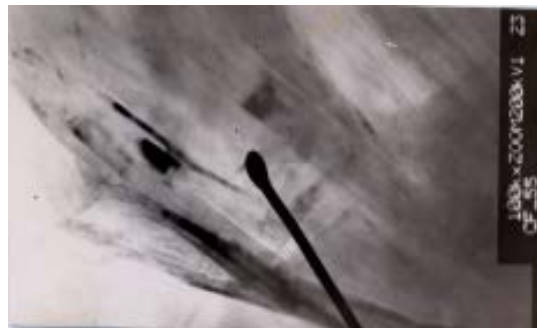
Fig. 4b: Structure of the high-modulus PAN fibre from TEM
