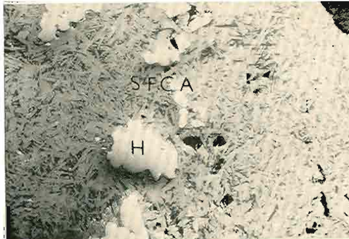
Fig. 4: Optical micrograph of sinter produced from 100% hematite ore at temperature of 1250°C in air x100 the microstructure consists essentially needle SFCA, dicalcium silicate and relict hematite (H)
