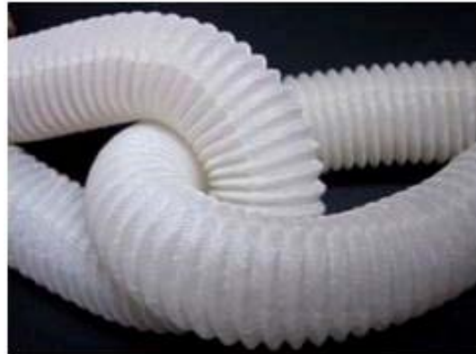
Fig. 4: Crimped tubes obtained with the new crimping process
