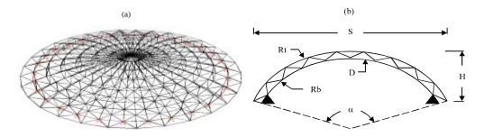
Fig. 2(a-b): General geometrical properties of models; (a) 3-d view and (b) Elevation
