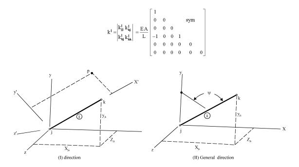
Fig. 1: An element of a truss
