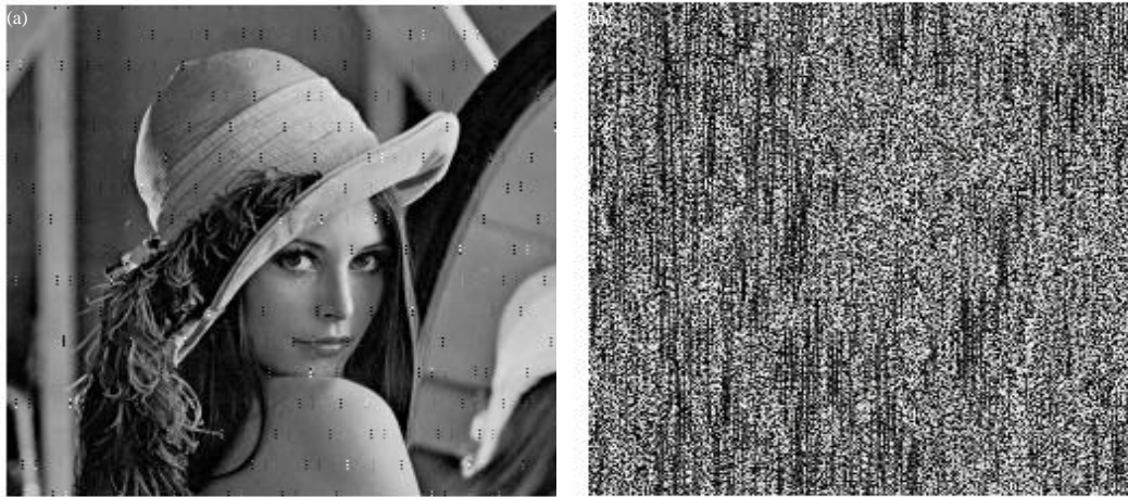
Fig. 10(a-b): Received image with E_b/N_0 = 10 dB \alpha = 2.3 and fiber length of (a) 10 and (b) 12 km
