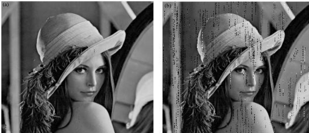
Fig. 13(a-b): Received image with E_b/N_0 = 9 dB, fiber length = 3 km and \alpha , (a) 2 and (b) 10
