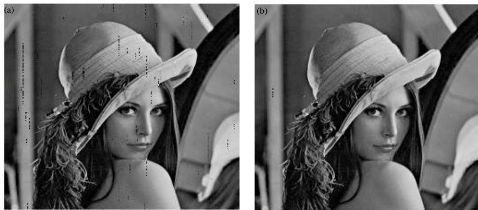
Fig. 5(a-b): Received image with fiber length = 800 m and E_b/N_o of (a) 7 and (b) 9 dB
